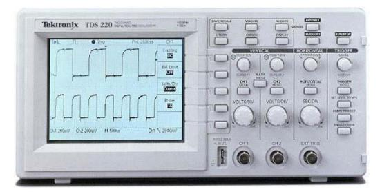
coupling: DC,AC DC= DC and AC+offset AC= only AC, blocking offset
