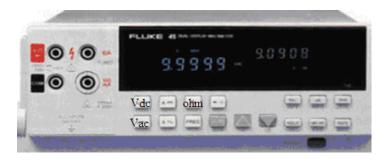
*Note*: Current measurement is done *in series* whereas voltage measurement is done *in parallel*.
